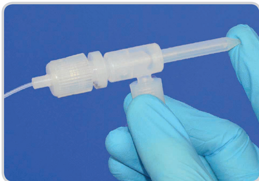
Clearing a blockage by backflushing a C-Flow – no need for tools or wires. Simply place a gloved finger over the tip while Ar nebulizer gas is flowing.
