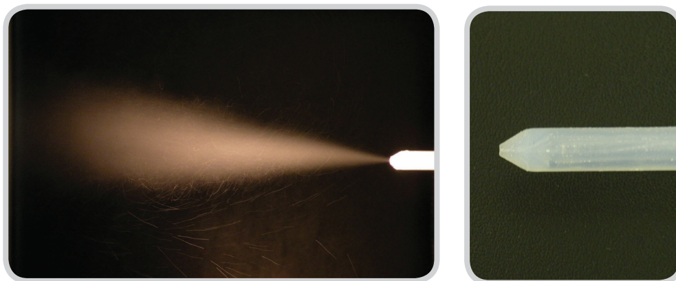
Aerosol of 25% w/v NaCl solution (left) and nebulizer tip (right) – both after four hours
