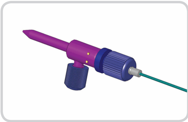
C700d Showing Uptake Line Connected
