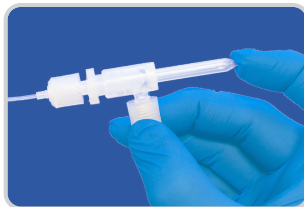
Clearing a blockage by backflushing a C-Flow – no need for tools or wires. Simply place a gloved finger over the tip while argon nebulizer gas is flowing.
