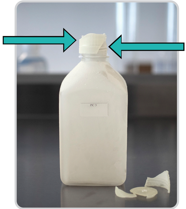
Figure 2: PC Closure Damage – Flat-on-Bottom Drop
