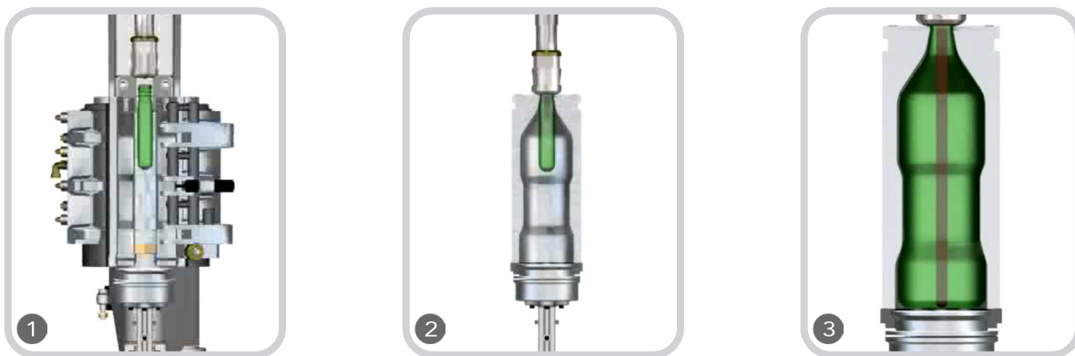
Figure 2: Stretch Blow Molding Process
